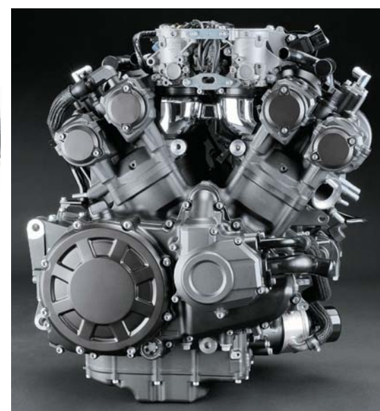
The engine retains the 70° V angle of previous versions
